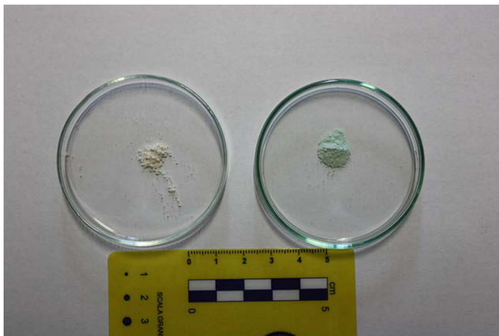
Fig. 3 Macroscopic picture of Na-PHI ( left side ) and Cu-PHI ( right side ) samples
