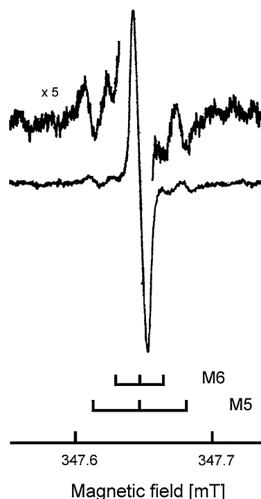
Fig. 10 EPR spectrum of the diamond, recorded with a microwave power of 0.01 mW and modulation amplitude of 0.05 G, exhibiting a new type of nitrogen paramagnetic centers M5 and M6 with extremely low splitting. Magnetic field is parallel to [100] crystal direction
