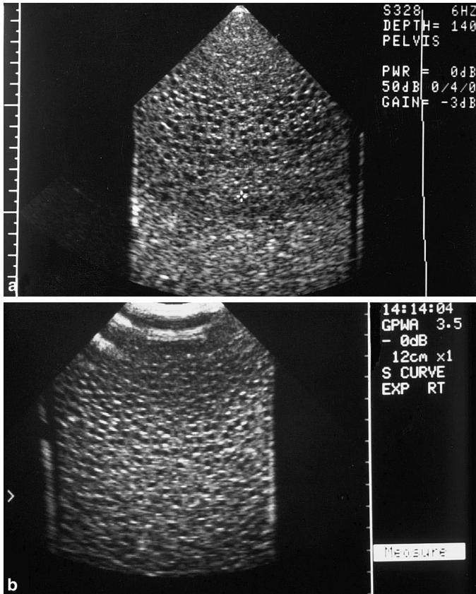
Fig. 2. a. Image of a phantom containing many small cystic structures obtained with an annular array transducer. An accurate representation of the cysts is obtained throughout the phantom. b. Image of the same phantom with a curved array transducer. Only the cysts lying in the focal zone are imaged clearly. The open arrowhead indicates the position of the focus.
