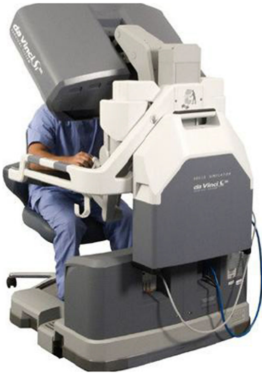
Fig. 5 Da Vinci ® Skills Simulator integrated with the da Vinci Si ® surgeon console
