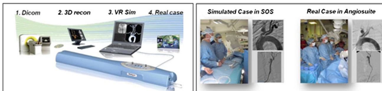
Fig. 7 Process of patient-specific rehearsal for carotid artery stenting using the Angiommentor Simulator ( left ). Example of its use as a rehearsal tool in the Simulated Operating Suite (SOS) before the actual case in the Angiosuite ( right ) (Imperial College London)
