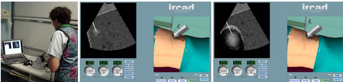
Fig. 3 Haptic Operative Realistic Ultrasonographic Simulator (HORUS), designed for ultrasound (US)-guided percutaneous interventions (printed with permission)
