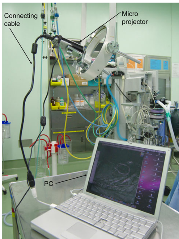
Fig. 1 Microprojector connecting with a personal computer was setting on the movable bar in the operation room
