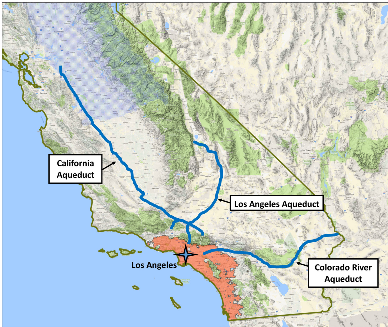
Fig. 1 Major conveyance systems for importing water to the Los Angeles metropolitan region. Two aqueducts, the Colorado River Aqueduct and the California Aqueduct, serve the greater Southern California region
