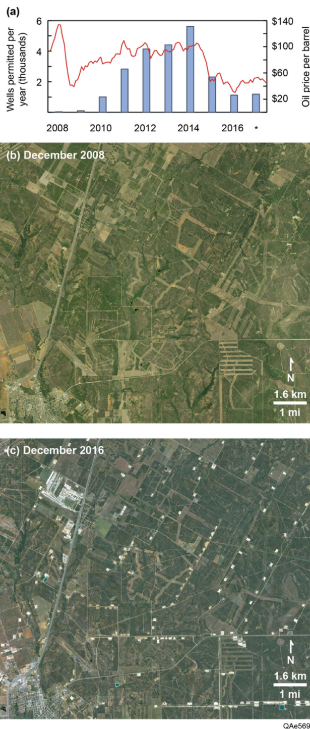
Fig. 1 Eagle Ford drilling and oil price history (a) and resulting landscape alteration from December 2008 (b) through December 2016 (c) for a representative portion of the play northeast of Cotulla, TX (southwest corner of images). Infrastructure construction includes roads, well pads, surface impoundments, storage facilities and railway transport terminal. Asterisks indicates well permitted by Texas Railroad Commission for Q1 and Q2 of 2017 (RRC 2018). Imagery: Landsat/Google Earth Pro. Oil price from EIA (2017c)
