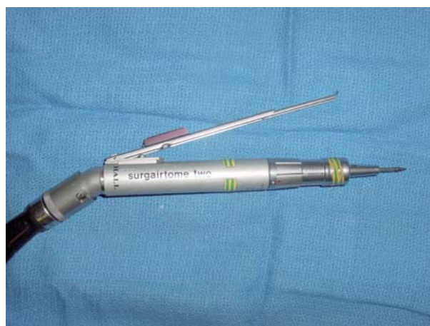
Fig. 4. Example of the gas-powered drill with a guarded 4-mm drill bit used to make cortical tunnels.
