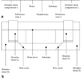
Fig. 1a, b Side elevation of presentation apparatus. a Standard experimental set-up. b Set-up allowing accommodation of additional concealed stimulus shoals to provide olfactory cues
