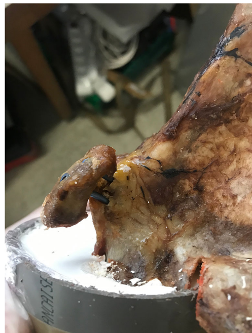
Fig. 4 One example of fixation failure: screws cut-out
