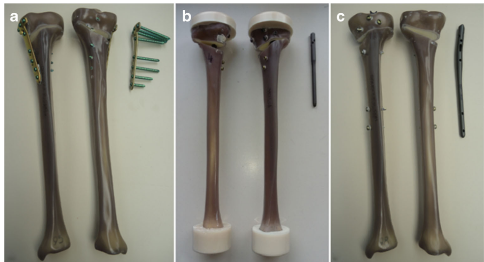
Fig. 2 Bone implant constructs with different fixation devices: a Tomofix®, b Targon PH® with grouting compound, and c Targon TX®. Because of an oblique projection, the osteotomy gap of image a seems to be smaller, but all gaps were performed identically by using a special fixation device
