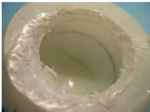
Fig. 3 Picture of an insert showing wear of the retention collar that led to intra-prosthetic dislocation
