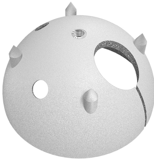
Fig. 1 Atlas IIIp is a modular cementless shelf feature with multi-perforated HA coated hemispherical titanium alloy (TiAl6V4) with four anti rotation spikes and a large central opening with a vertical split in the lower part of the shell
