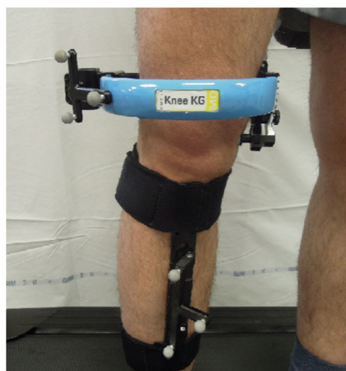
Fig. 1 Anterior view of a right knee fitted with the Knee-KG™ tracker system. Secure fixation on the thigh and calf minimises skin-motion artifact
