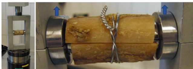
Fig. 2 Test setup. Cortical half shells mounted on cylindrical metal bars with one 1.5mm wire cerclage double looped around the bone, tightened and closed by a twist. Cyclic loading (blue arrows) tends to separate the half shells against cerclage tension. Wire and cable cerclages were investigated. On the left, the complete test setup-frame is shown with cylindrical metal bars, mounted specimen, load cell at the bottom and the actuator on the top
