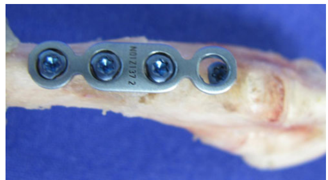
Fig. 5 In many cases, the interlocking mechanism fails by a deformation of the plate hole. Thus, the screw could slide through the hole
