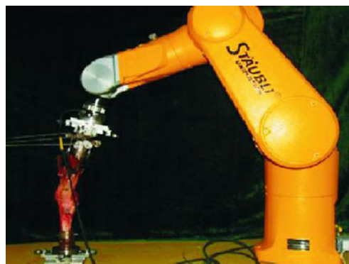
Fig. 2 Knee-test model of the multiplane load based on the robot. Activity of a knee specimen was simulated for testing using the Staubli robotic/UFS testing system
