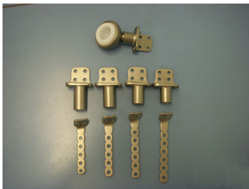
Fig. 1 Components of a typical prostheses are shown. The set typically consists of three components: iliac fixation components with variable-length bush, acetabular component and pubic connection plate. All components are made of titanium
