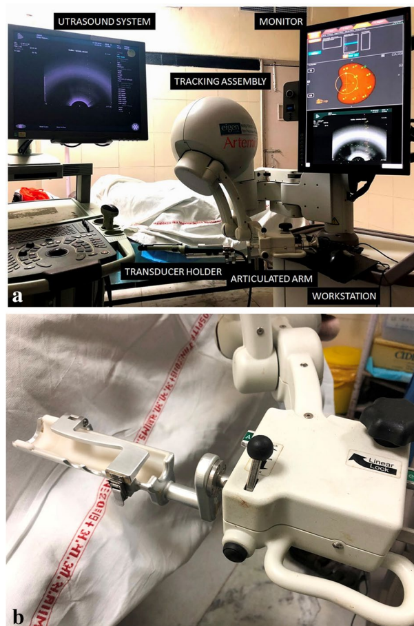
Fig. 2 a The Artemis MRI–TRUS fusion biopsy platform (Eigen, Grass Valley, CA, USA). b The system has a transducer holder into which the probe can be placed and locked. The holder is attached to an articulated arm which enables mechanically stabilized freehand sweep. The arm is connected to the tracking assembly, which enables real-time probe tracking and navigation. A monitor and workstation are provided as the operator interface
