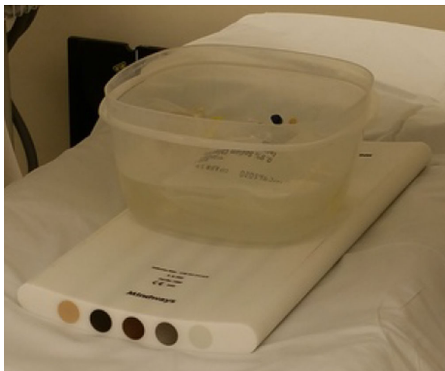
Fig. 1. In-house constructed phantom, consisting of 17 cm × 17 cm plastic container with water, a saline solution filled bag, and ultrasound gel. This is placed on top of a commercial CT head calibration phantom (Mindways, Austin, TX USA).
