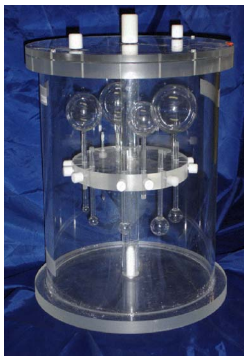
Fig. 1 Phan1 as used for evaluation of the contrast-oriented algorithm comprising ten fillable spheres of different diameters
