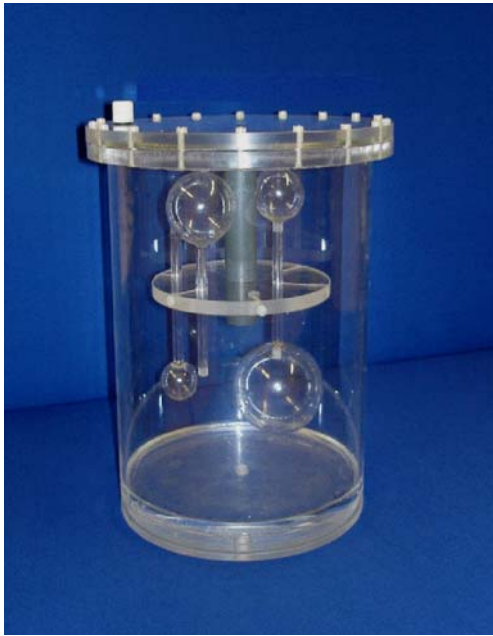
Fig. 2 Phan2 as used for validation of the contrast-oriented algorithm comprising four fillable spheres of different diameters
