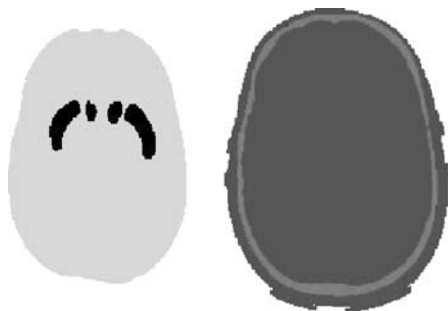
Fig. 1 A central slice of the activity distribution ( left ) and the attenuation map ( right ) of the striatal phantom. The striatal nuclei can be observed in the activity distribution
