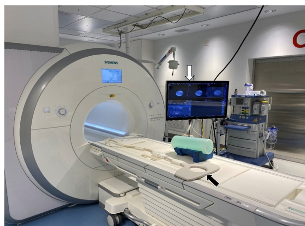
Fig. 1 Interventional MRI suite. The interventional MRI suite includes a wide-bore 3.0 T MRI scanner (Magnetom Skyra, Siemens Healthcare), an MRI-conditional in-room monitor (white arrow) for scanner control and image display, and an interventional MRI coil (black arrow)
