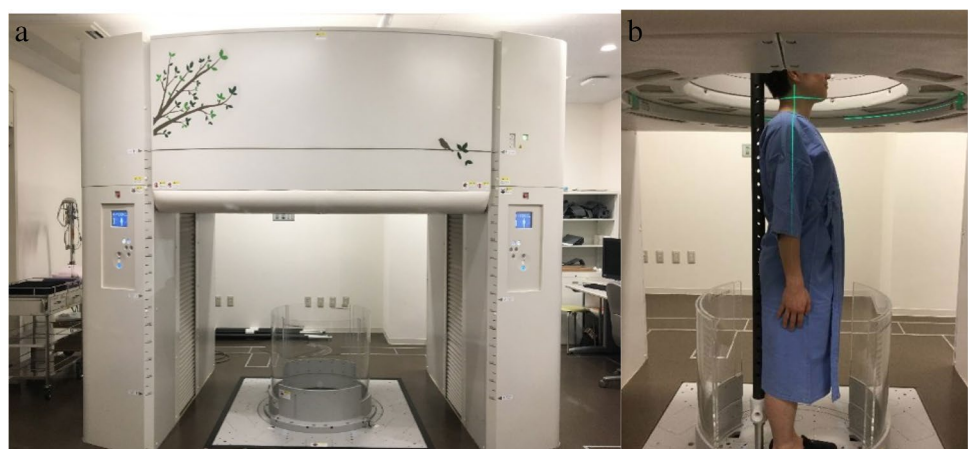
Fig. 10 Photograph of 320-row-detector upright CT. a Image shows the upright CT with gantry in the up position. b The subject standing in the gantry
