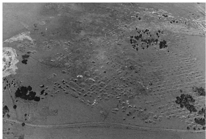
Fig. 5 Pattern of collapses at the surface due to void migration in bord areas
