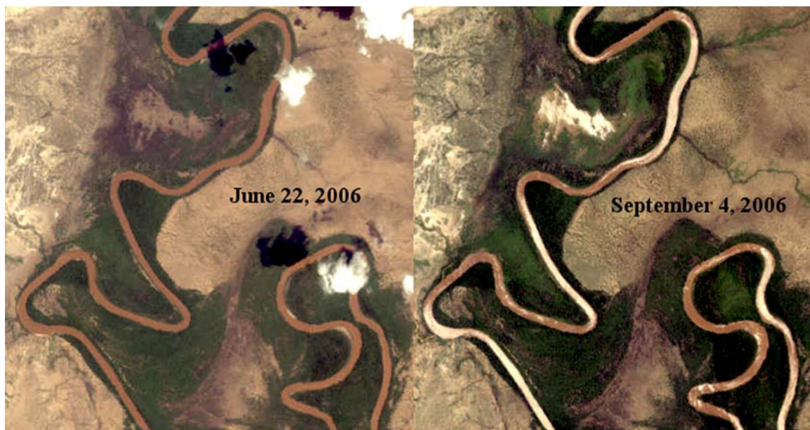
Fig. 7 Images showing the accumulation of sediments in the lower part of the meander belt after the flood in 2006
