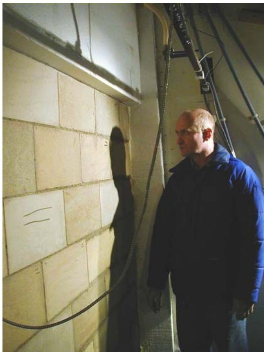
Fig. 4 Inspection of test wall in climatic simulation test chamber
