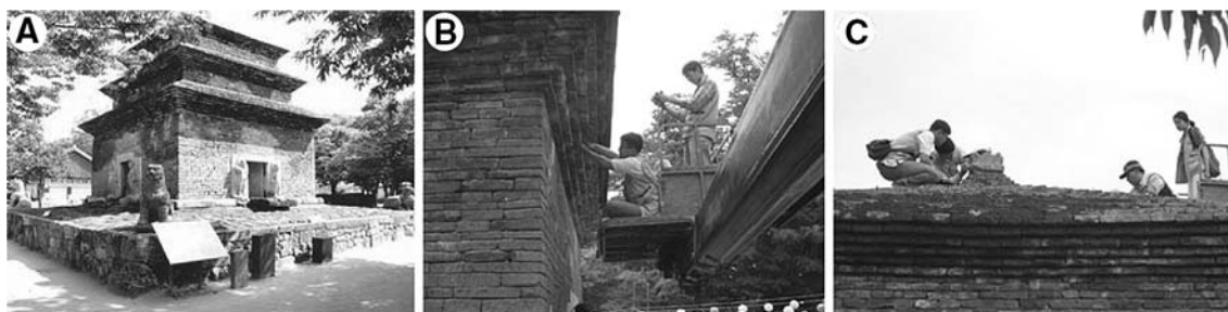
Fig. 2 Field occurrences of the stone pagoda in the Bunhwangsa temple. a General view from the southwestern side. b Stalactite-like white precipitates collected from northern body rocks of the
