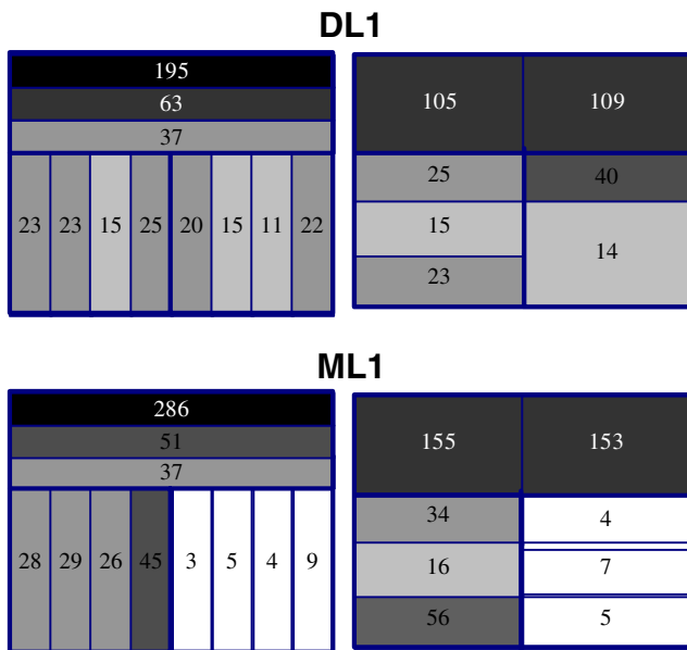
Fig. 13 Final salt distribution in specimens DL1 and ML1 (kg NaCl/m 3 open porosity in the stone). Both halves of either specimen are in side-view (Fig. 4)
