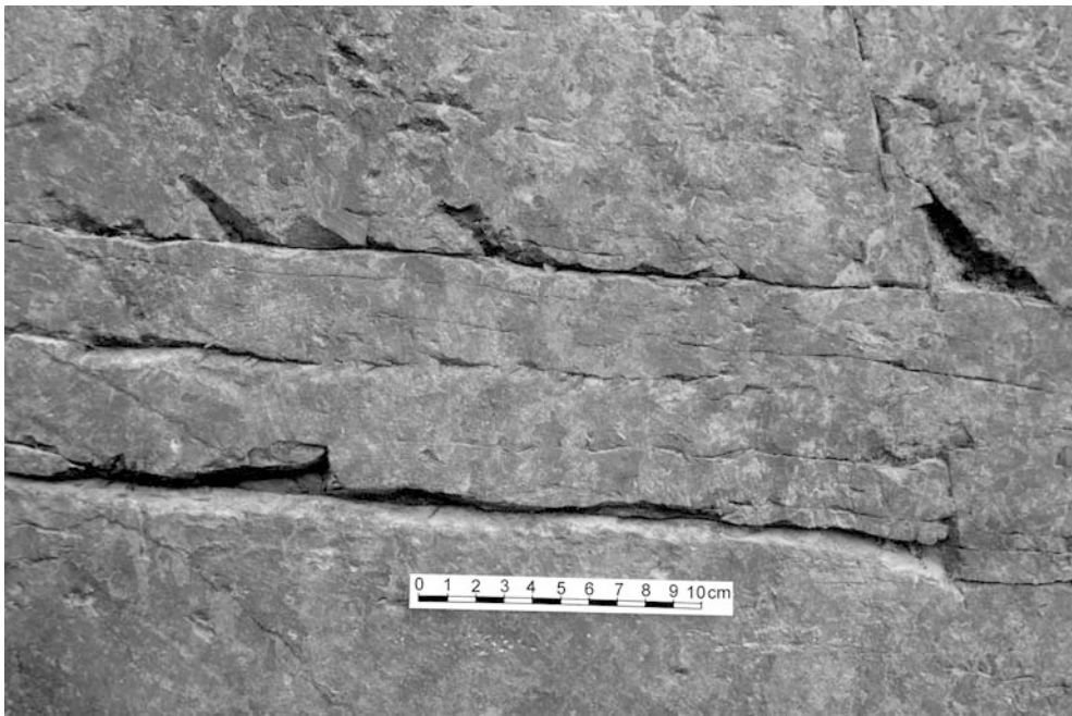
Fig. 10 Weathering form “splitting up (Xv)”
