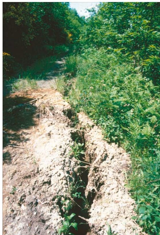
Fig. 19 Approximately 10-cm-wide tension fracture in the pyroclastic covers
