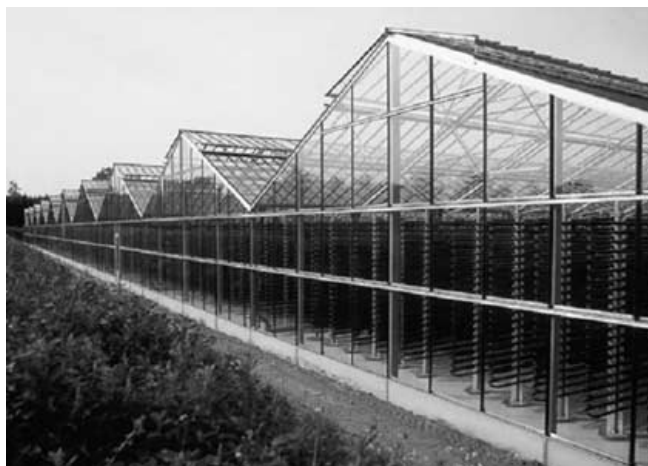
Fig. 5 700 m 3 glass tube photobioreactor producing Chlorella biomass
