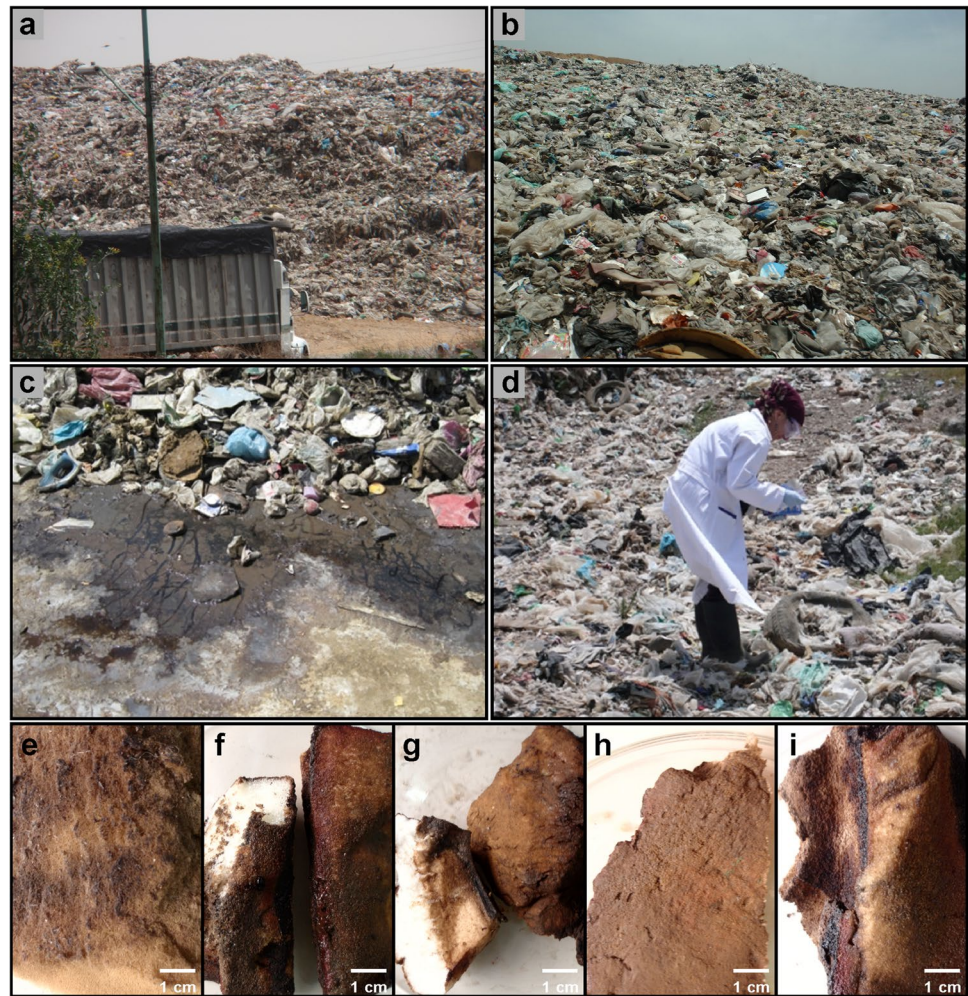
Fig. 1 Foam samples collect at El Bordo Poniente landfill (near Mexico City). a Size comparison between a truck and the garbage piles at El Bordo Poniente landfill. b A general landscape. c Landfill leachate drained from garbage piles as a result of rotting and decomposition of organic matter. d Manual collection of samples. e–i Foam samples collected at different microenvironments and used as inocula for enrichment selection in MM-PolyLack. e BP1, f BP2, g BP4, h BP5, and i BP7
