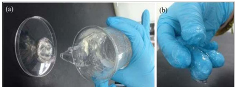
Fig. 3 a Highly viscous and b sticky GG suspension produced using 1.50 g GG (With Courtesy to paper by Ismail et al 2018)
