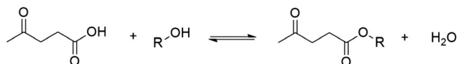
Fig. 1 Scheme of the esterification of levulinic acid (LA) with alcohols ( R = \text{CH}_3 or \text{CH}_2\text{CH}_3 or (\text{CH}_2)_3\text{CH}_3 ). Provenance and purity of compounds used in this study are listed in Table S1
