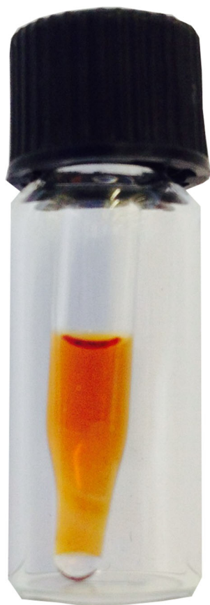
Fig. 5 Yellowish oil, containing low-molecular-mass aromatics, obtained after enzymatic depolymerization of OrganoCat lignin
