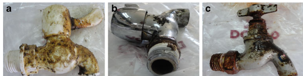
Fig. 2 Tap samples with three different materials: PVC (a), stainless steel (b), and cast iron (c) taken from one household
