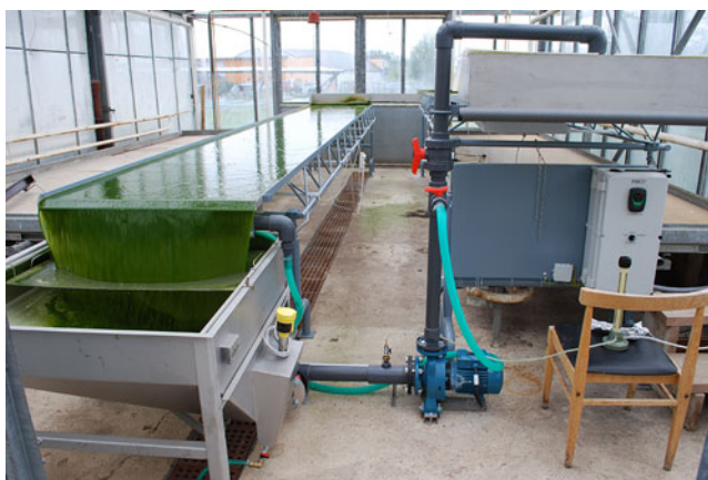
Fig. 5 Thin layer PBR in a greenhouse of the Institute of Botany, Třeboň, August 2010
