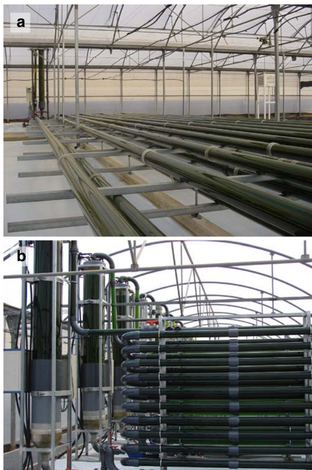
Fig. 1 a 4,000-L two-loop horizontal tubular photobioreactor growing S. almeriensis (Fernández-Sevilla et al. 2005). b A later redesign is the 10-unit fence-type configuration (Fernández-Sevilla et al. 2008) totaling to 28,000 L. Both systems are built inside a greenhouse at the “Las Palmerillas” agricultural research station (El Ejido, Almería, southern Spain, with permission of Prof. J. Pérez Parra, Fundación CAJAMAR)
