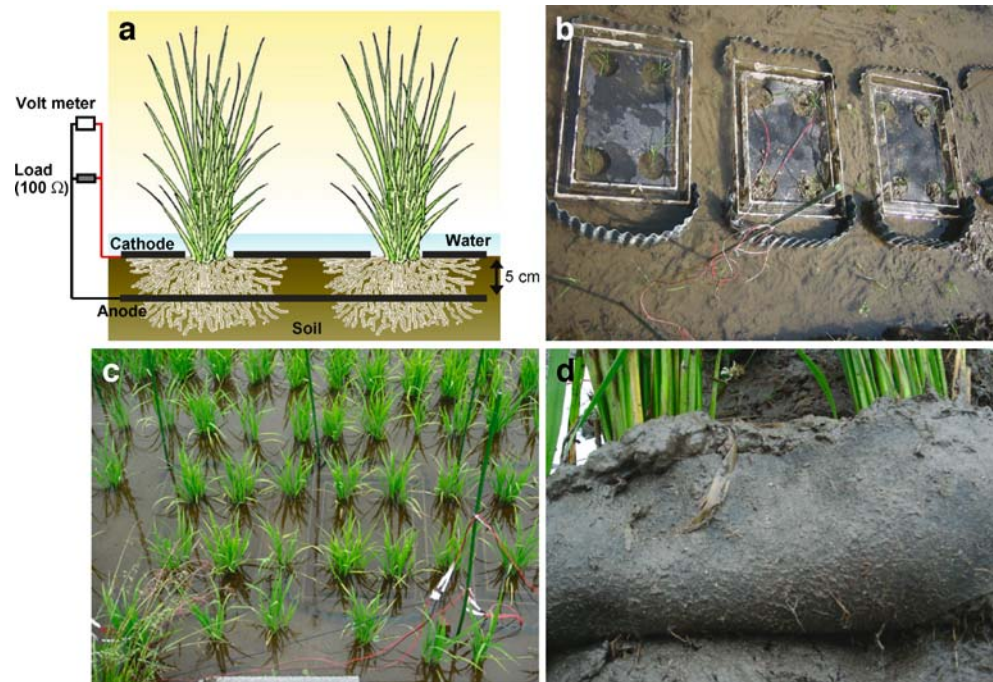
Fig. 1 The paddy-field power-generating system. a Schematic illustration showing positions of the anode and cathode relative to rice plants. b The power-generating system immediately after starting the operation (May 16th). c The power-generating system in operation (June 23rd). d The backside of an anode graphite felt showing that rice roots penetrated the anode (August 7th)
