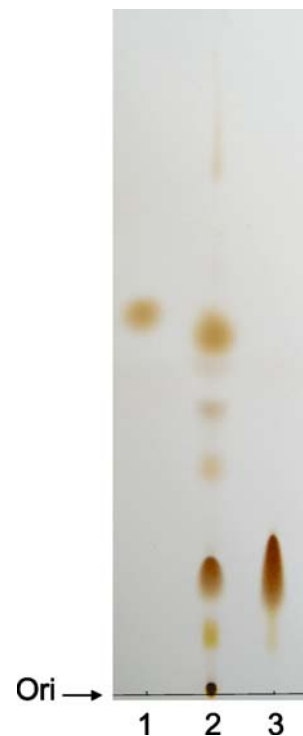
Fig. 2 Thin-layer chromatography of the crude extract and purified product from the bioconversion of palmitoleic acid by PR3. lane 1 palmitoleic acid, lane 2 crude reaction products, lane 3 purified product. Running and developing conditions are given in the Materials and methods section
