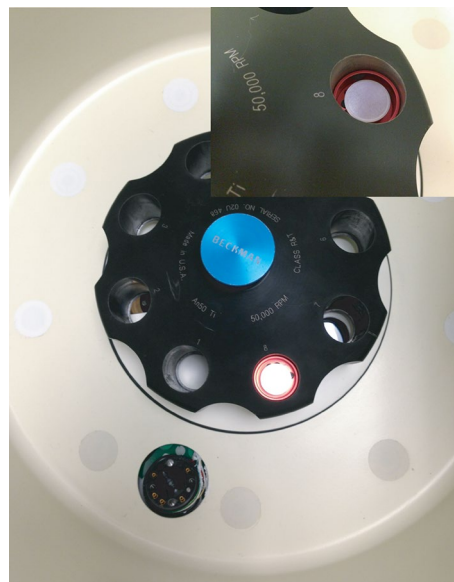
Fig. 1 Picture of iButton positioned top of the counterbalance in an 8-hole rotor for determining the temperature of a resting rotor. Reproduced from (Ghirlando et al. 2014)
