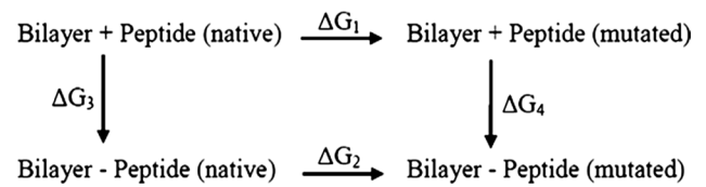
Fig. 1 Thermodynamic cycle for computing the relative binding free energies of two peptides (native and mutated) to a bilayer
