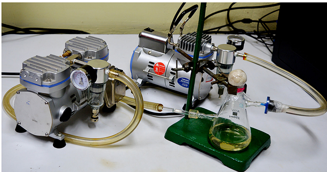
Fig. 2 Experimental setup for trapping of volatiles emitted by the G. candidum PF005 fungus in the Porapak Type Q polymer, as described in the “Materials and Methods” section
