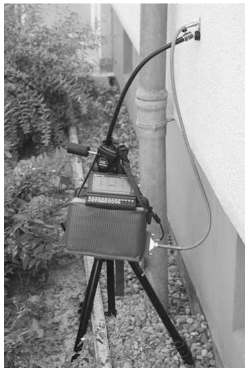
Figure 1. Fluorometric measurement of photosynthetic efficiency in situ of an algal community growing onto a building facade in Rostock (Germany) using a PAM 2000 (Walz, Germany). The light conductor was always fixed on a tripod (Manfrotto, Italy) at a constant angle of 60°.
