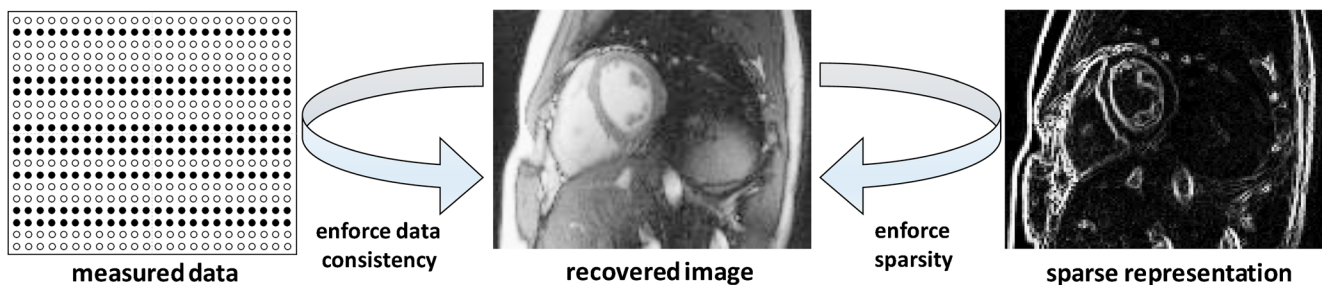
Fig. 3 Depiction of a typical compressed sensing method employed for MRI recovery. Under this approach, the image is iteratively recovered by enforcing both data consistency and sparsity constraints. Because most images are not sparse in their ambient domain, a sparsifying transform,
