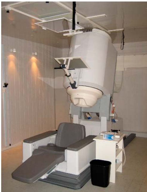
Fig. 1 CHOP's 275-channel whole-head MEG system in its magnetically shielded room
