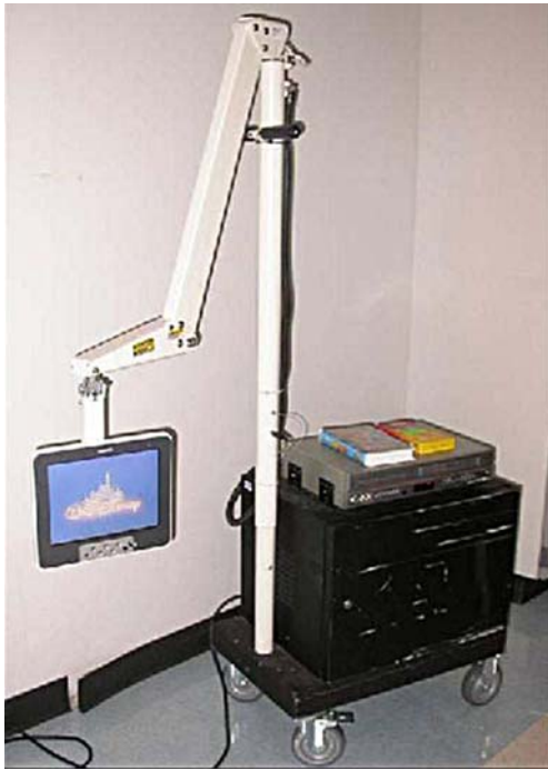
Fig. 3 DVD player mounted on a movable cart, with the screen on a movable arm is particularly helpful in CT where the patients may be imaged prone, supine, feet-first or head-first
