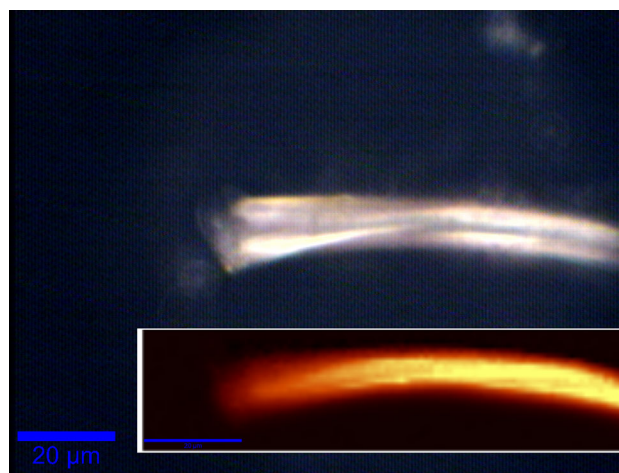
Fig. 2 White light micrograph of a PET fiber. Inset Raman chemical image of the fiber, for the corresponding Raman spectrum, see Fig. 3 (spectrum 2)
